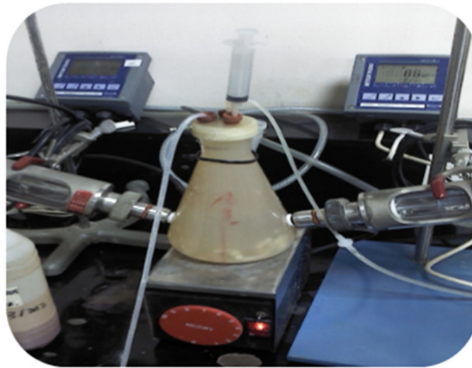
Figure 3. Photo illustrating the bioreactor setup with ORP and pH sensors.
